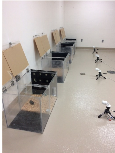
Figure 1. Picture of 4 of the 8 clear box trial containment units (lids remained open during trials) with monitoring cameras. Note the clear plastic partition that divides each unit where food and mate incentives were placed in attempt to encourage the mouse to escape to the other side of the partition.
