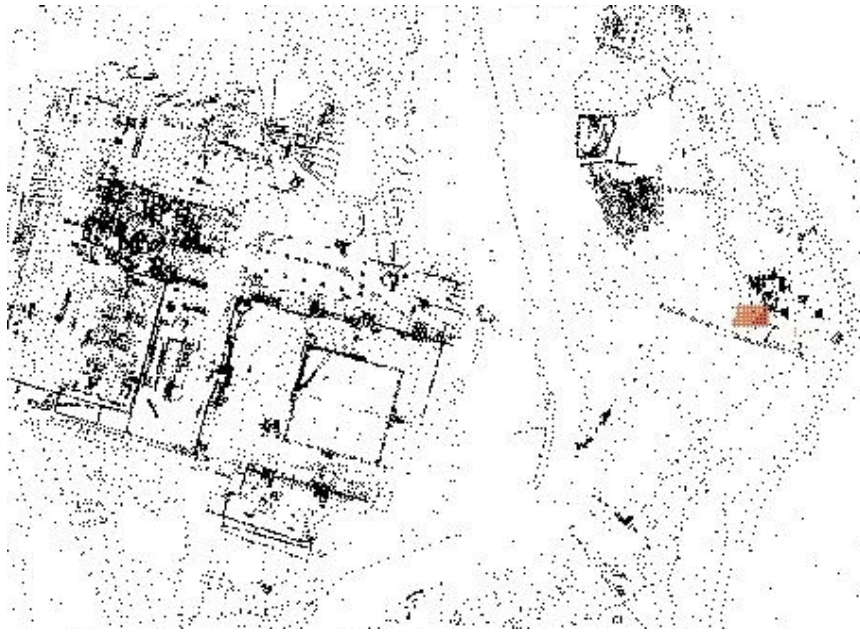
Figure 6.3: Chavín de Huántar, location of La Banda excavation units in red. These points were recorded with a theodolite and the map was made from the accumulation of thousands of data points. The river is blank and the La Banda units are to scale. The map was made by Dan Contreras and John Rick using a Leica Total Station.
