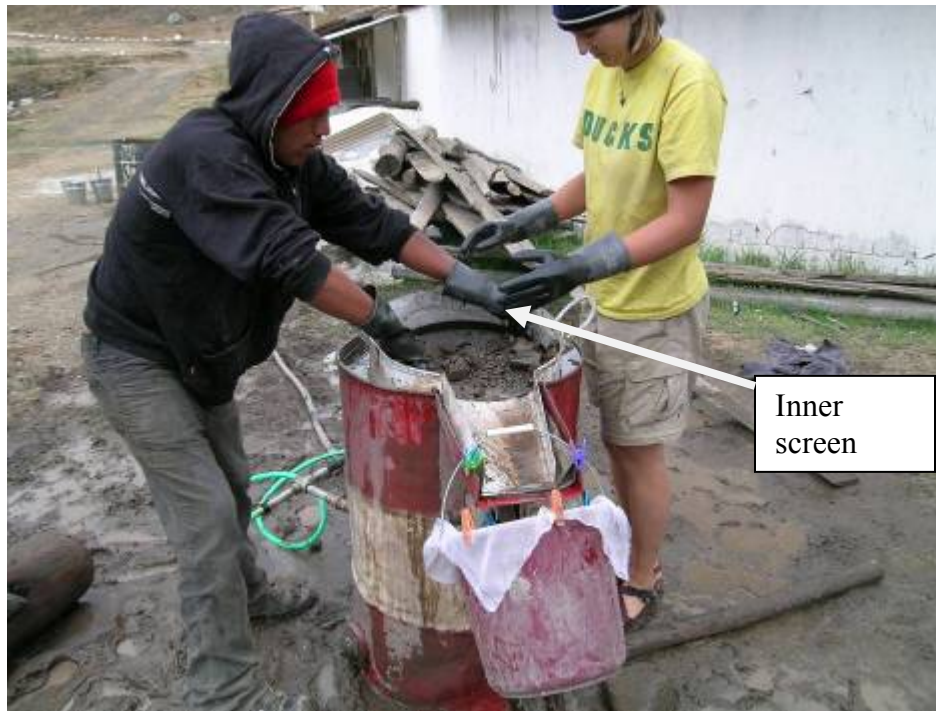
Figure 7.2: Flotation machine and component parts
