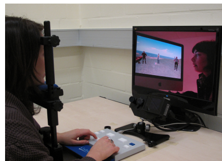
Figure 2: Eyetracking setup: Participants watched the video on the screen, then pressed a button in response to the template.
