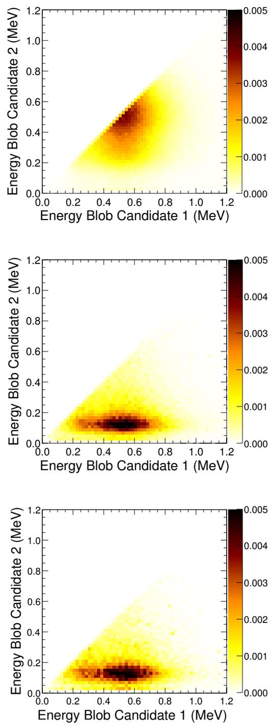
**Figure 6.** Probability distribution of  $0\nu\beta\beta$  (top panel),  $^{208}\text{Tl}$  (centre) and  $^{214}\text{Bi}$  (bottom) events in terms of the energies at the end of the tracks. The blob candidate labelled as ‘1’ corresponds to the more energetic one.
