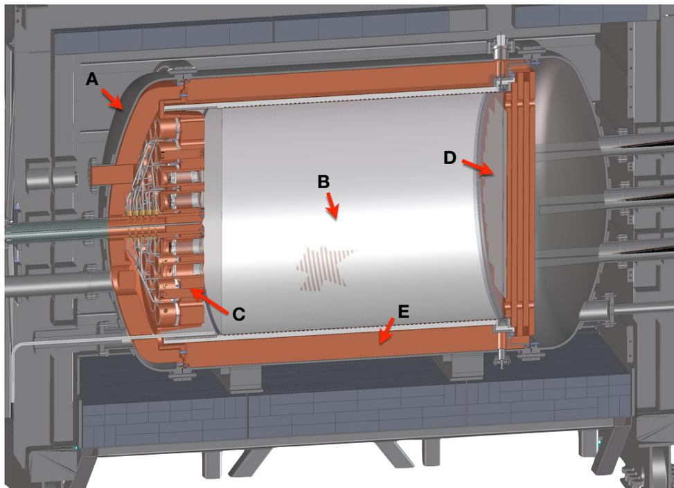
**Figure 2.** Cross-section view of the NEXT-100 detector inside its lead castle shield. A stainless-steel pressure vessel (A) houses the electric-field cage (B) and the two sensor planes (energy plane, C; tracking plane, D) located at opposite ends of the chamber. The active volume is shielded from external radiation by at least 12 cm of copper (E) in all directions.
