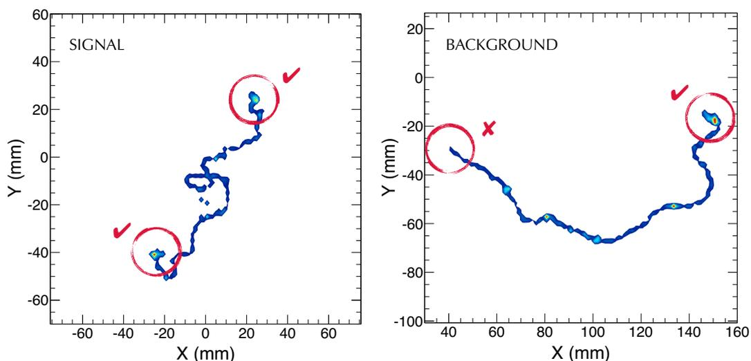
**Figure 3.** Monte Carlo simulation of signal ( $0\nu\beta\beta$  decay of  $^{136}\text{Xe}$ ) and background (single electron of energy equal to the  $Q$  value of  $^{136}\text{Xe}$ ) events in gaseous xenon at 15 bar. The colour scale codes the energy loss per path length. The ionization tracks left by signal events feature large energy deposits (or *blobs*) at both ends.
