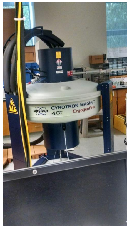
Figure 3.3: The gyrotron magnet used in these experiments at the Materials Research Lab at UCSB.
