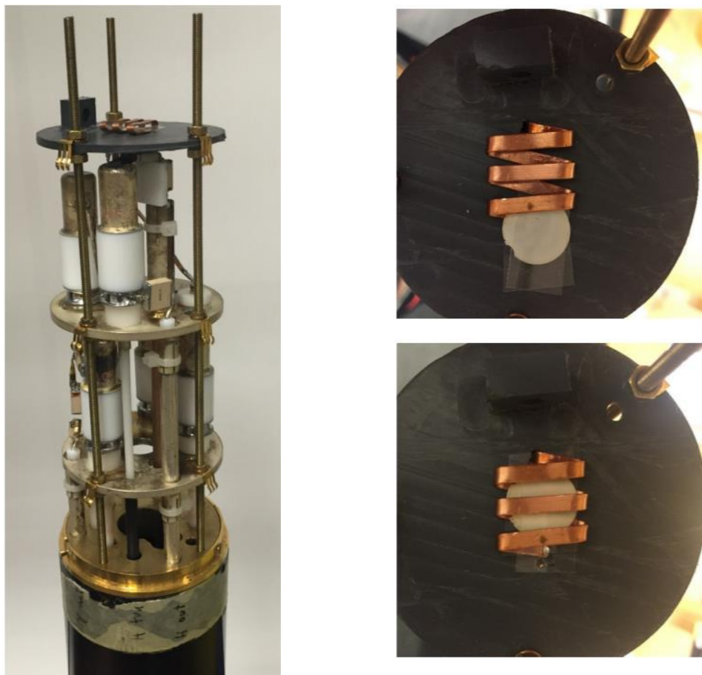
Figure 2.2: Flat coil NMR probe and a close-up of the AAO template being inserted into the flat coil.
