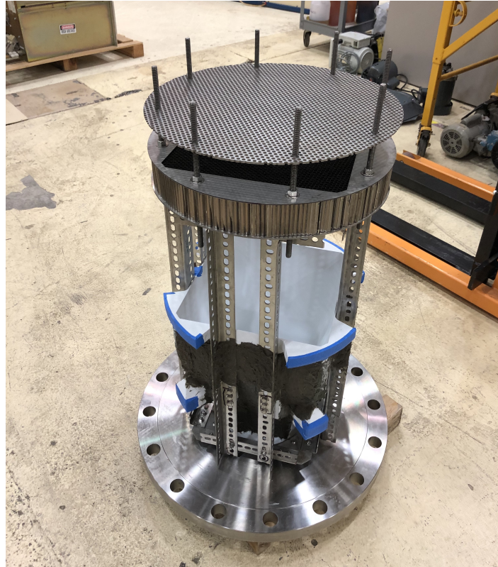
Figure 3.6: The flow conditioning insert consists of (from top to bottom) two perforated stainless steel plates (only one shown), a honeycomb, a settling chamber (walls not shown) and a 4:1 3D printed contraction. The assembly is supported by a stainless steel frame. Shown during a fit check, it is sitting atop the stainless steel flange that is used to cap the outlet end of the contraction tank.
