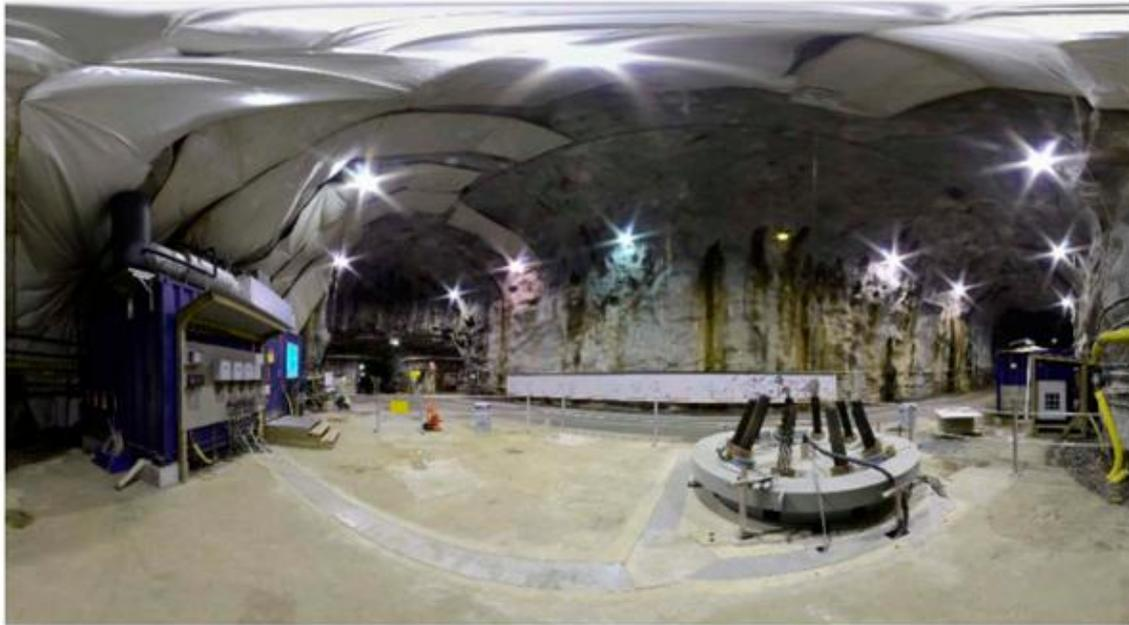
**Figure 14. A panoramic view of the Large-scale gas injection test (Lasgit) 420 m below ground at the Äspö Hard Rock Laboratory in Sweden (from Cuss et al. 2022). The blue container on the left housed the artificial hydration and gas injection systems which were connected into the borehole along channels cut into the gallery floor. The cap and rock anchors of the deposition hole can be seen into the centre right.**
