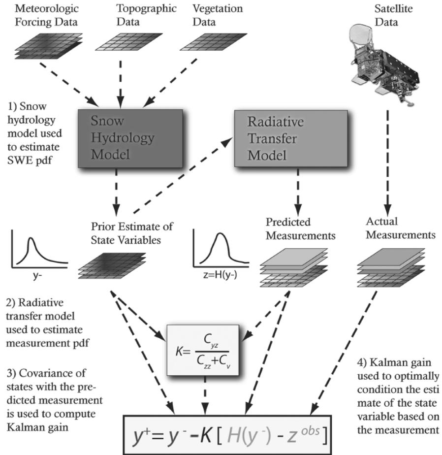
**Figure 2. Schematic of EnKF methodology used for snowpack characterization. The snow model and radiative transfer model are used to generate prior distributions of predicted model states and measurements and to compute the Kalman gain  $K$ . The actual observations are used along with the Kalman gain to update the prior states.**
