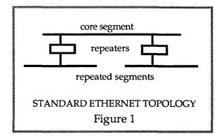
The repeaters may be local or remote. Remote repeaters are pairs of repeaters interconnected with up to 1000 meters of optical fiber cable. This is typical of the existing LBLnet. The maximum overall length of a standard Ethernet is then calculated as three 500 meter segments and 1000 meters of repeater fiber for a total of 2500 meters (actually 2800 meters if the six possible 50 meter transceiver cables are added in).
