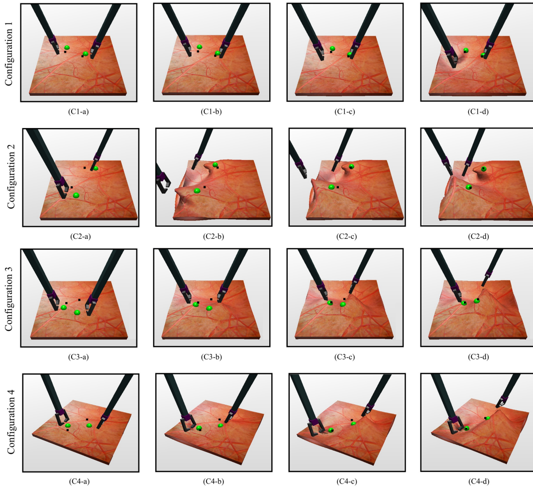
Figure 5.4: Example successful policies. Four configurations (C1-C4) are displayed for representative progressing actions during testing episodes from (a) initialization to (d) task completion . Each configuration represents a different set of initial TTPs, IDPs, and TGPs. Additionally, in (C4), the camera configuration is changed. In order to maintain simulation stability, it was necessary to manipulate TGPs via simulated springs with low stiffness connected to the graspers. As such, small gaps between graspers and the tissue are observable for large deformations.
