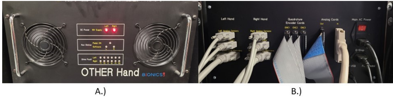
Figure 3.10: The electronics box containing the power supplies, motor controllers, and wire routing PCBs. A.) Front panel. B.) Rear panel.
