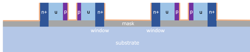
Figure 3.13 Metal contacts deposited onto island sidewalls and metal pads deposited onto the mask (salmon color).
