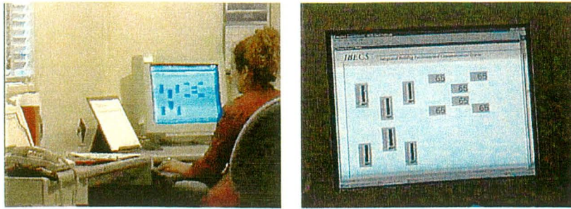
Figure 6. Left image shows occupant using IBECS to change the dim levels of the overhead lights using the computer. The right image is a closeup of the IBECS control screen. Note the six "sliders" on the left portion of the image each corresponding to a separately controlled ballast.
