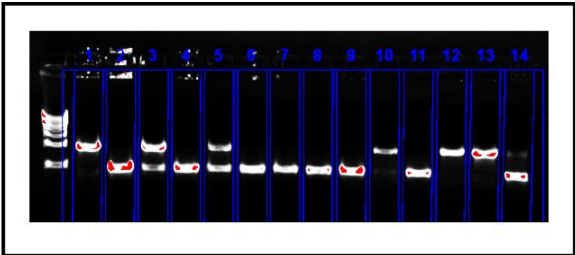
Figure 3-2: Gel electrophoresis of amplified genomic fragments from the three primer system. The sample used a 1 kb ladder with three possible results in each sample lane: 1 kb, 2 kb, and both bands.
