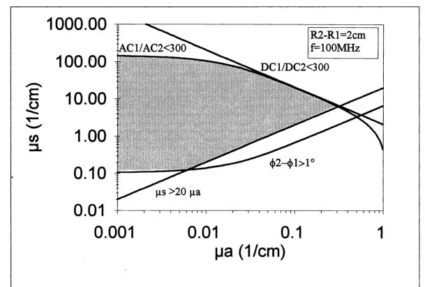
Fig. 5. Values of  $\mu_a$  and  $\mu_s$ ' that can be measured with our instrument. The conditions discussed in the text define the measurable region in the  $\mu_s$ ' –  $\mu_a$  plane, which is shown shaded. Note that the typical values of  $\mu_a$  and  $\mu_s$ ' in tissues  $(\mu_a \sim 0.01-0.1~\text{cm}^{-1}, \mu_s \sim 1-100~\text{cm}^{-1})$  fall inside the measurable region.
