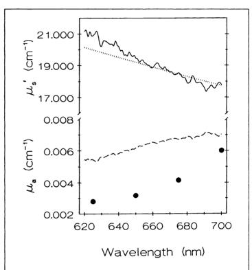
Fig. 2. Scattering (solid line) and absorption (dashed line) coefficients spectra of the Liposyn solution containing no methylene blue. The two spectra are compared, respectively, with  $\mu_s$ '( $\lambda$ ) predicted by van Staveren *et al.* (dotted line) and with several values of  $\mu_a(\lambda)$  for water known in literature (symbols).
