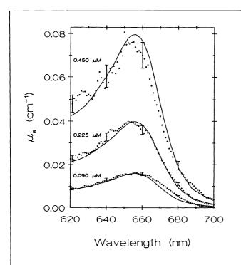
Fig. 3. Quantitative comparison between methylene blue (MB) absorption coefficient spectra measured in the strongly scattering medium by the LED technique (symbols) and in a non-scattering regime by a spectrophotometer (lines). The spectra correspond to MB concentrations of 0.090, 0.225, and 0.450 µM as labeled. Errors bars for the experimental data relative to the strongly scattering medium are shown every 20 nm.
