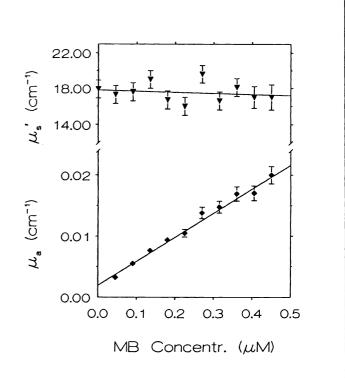
Fig. 4. Dependence of the values of  $\mu_{a}$  and  $\mu_{s}$  at 680 nm on methylene blue concentration. The straight lines are obtained by a weighted least square method. When the error bars are not displayed they are on the order of the symbol dimensions.
