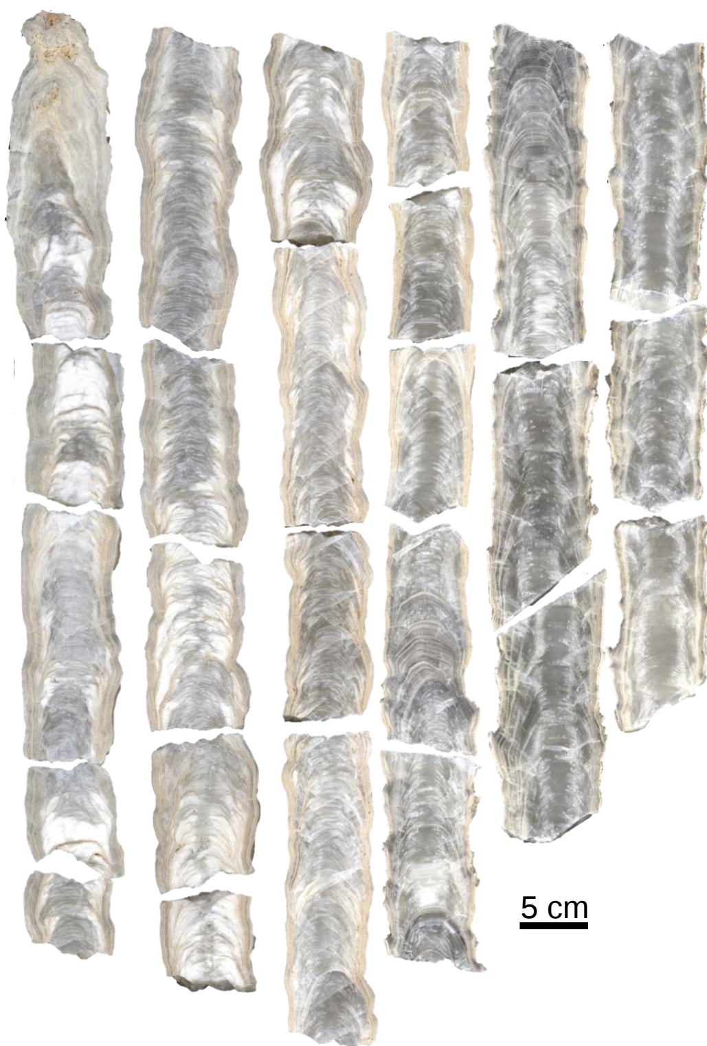
Figure 1.2. Scans of stalagmite HH-1. See Appendix A for image with U-Th dates labeled.
