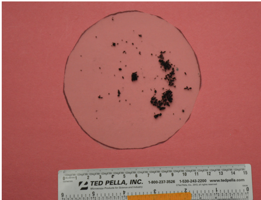
77 Figure S3. Image of aged top-load Jacket D 333 \mu m filter showing the pilling effect of smaller 78 fibers, causing them to catch on the larger filter.
