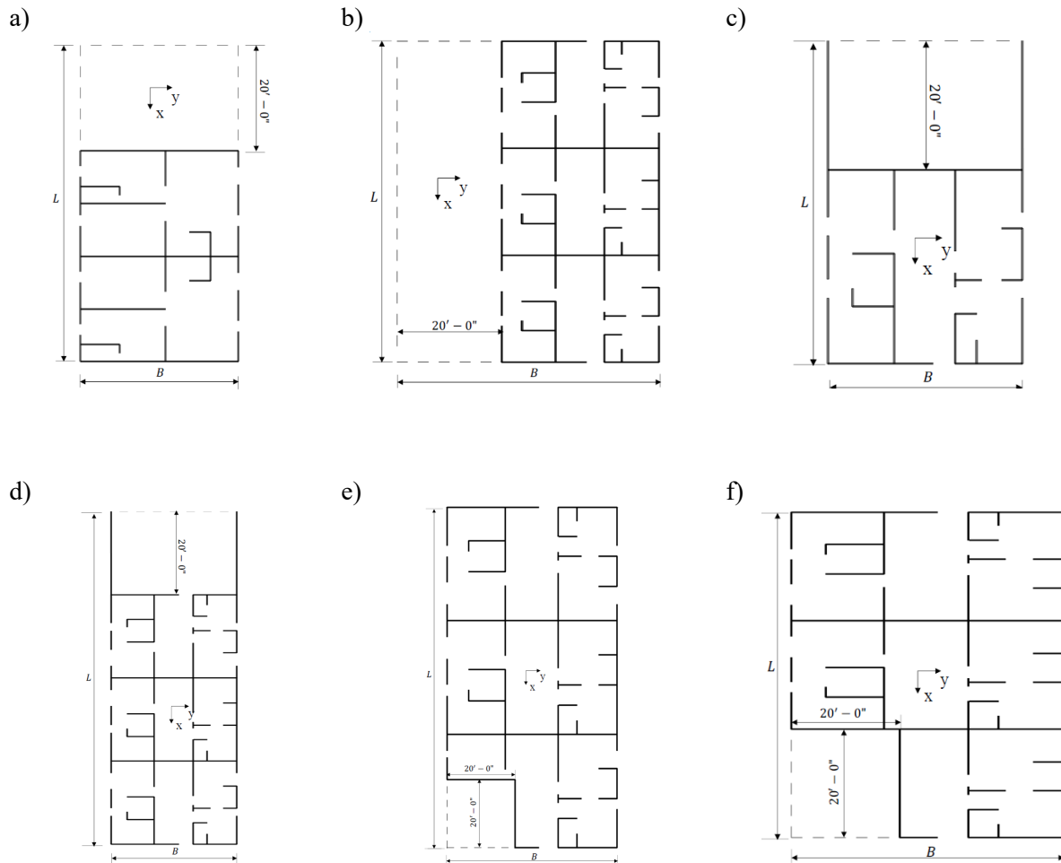
Figure 5.11. The first floor plan including the wood-frame walls for first-story wall layout categories a) L1, b) L2, c) L3 (L=50'), d) L3 (L=80'), e) L4 (L=60'), and f) L4 (L=100') adopted from Yi (2020)
