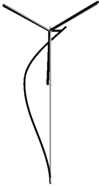
Figure 2.14: OpenSees Model II 2 nd side-to-side mode (12.1 Hz)
