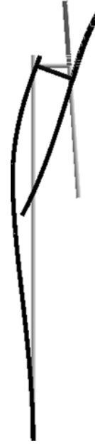
Figure 2.13: OpenSees Model II 2 nd fore-aft mode (9.7 Hz)
