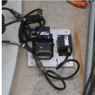
Figure 4.4: 3 Epi-Sensor ES-U units mounted to capture three orthogonal axes
