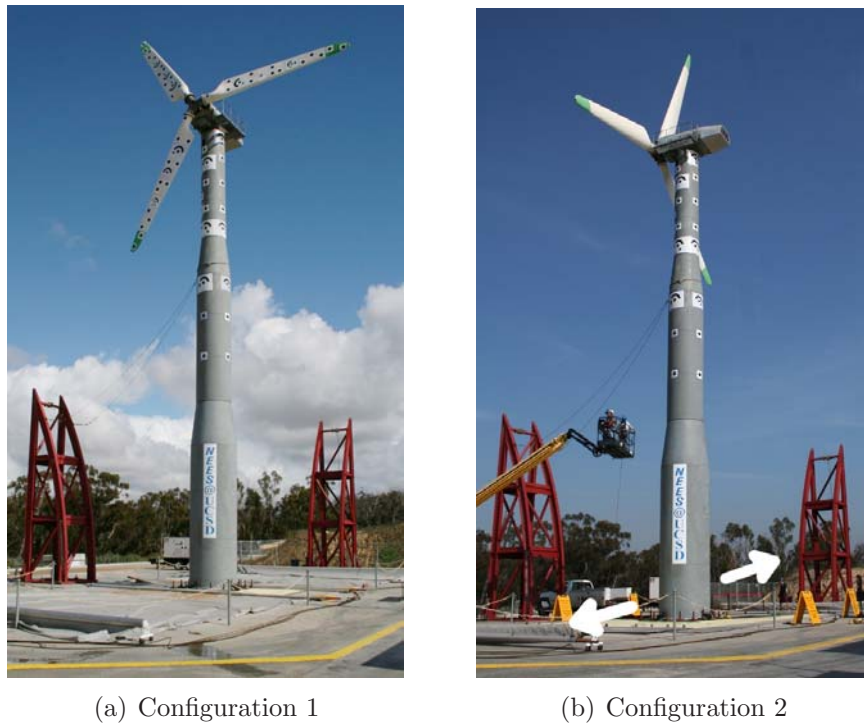
Figure 3.1: Wind turbine on the LHPOST (arrows indicate direction of shaking)
