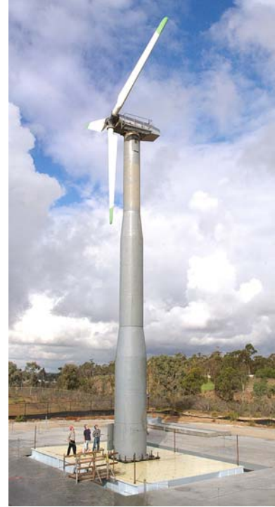
Figure 2.2: Wind turbine mounted on the outdoor UCSD shake table
