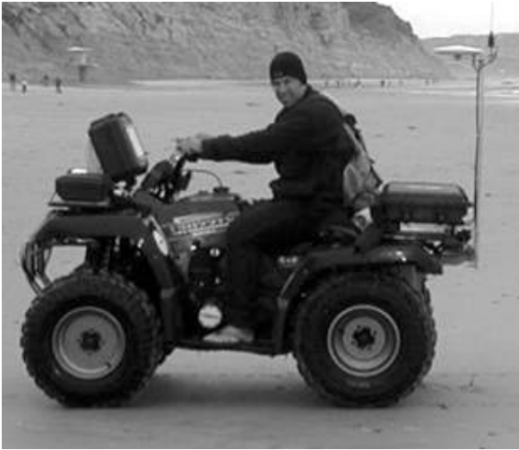
Figure 6. GPS-navigated all-terrain vehicle for dry beach surveys.
