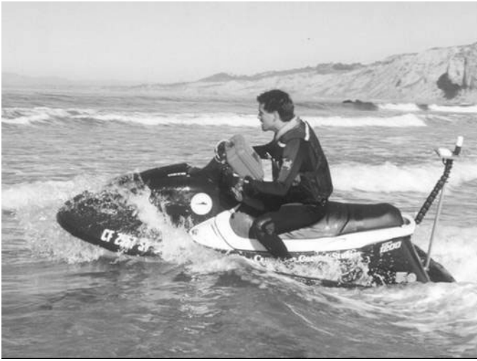
Figure 7. GPS-navigated JetSki for underwater surveys
