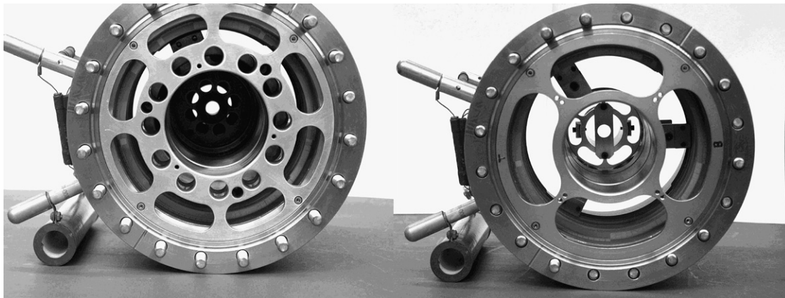
Fig. 3. Old and new extraction assemblies, showing the larger pumping apertures of the new design.
