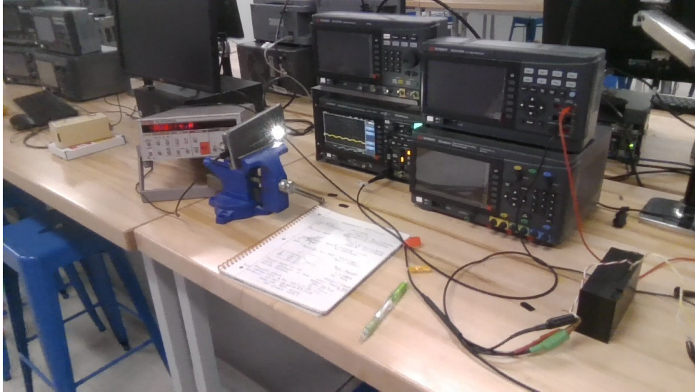
Figure 3-16: Experimental setup for initial design - The distance and position of the flashlight and the TIA is kept fixed. The oscilloscope is disconnected to record current readings. Then, the picoammeter is disconnected while the oscilloscope is connected, and the TIA is switched on to record the output voltage.
