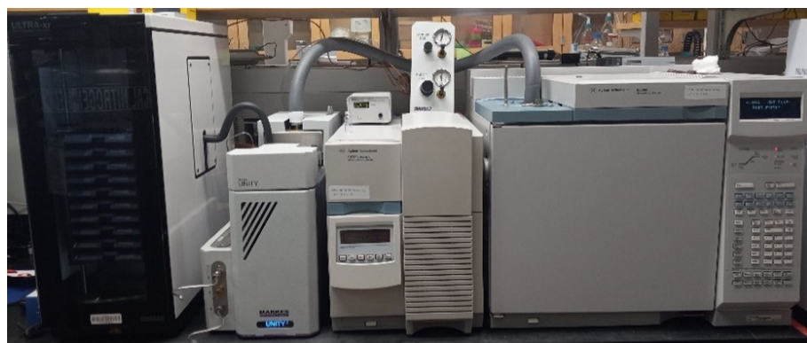
Figure 5. Equipment used for Thermal Desorption-Gas Chromatography-Mass Spectrometry analysis.
