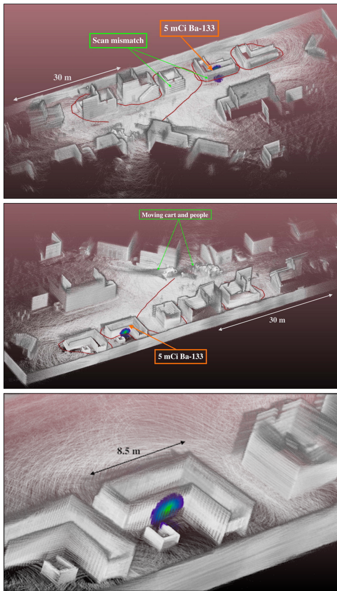
Fig. 6. (Color online) Final MLEM reconstruction (10 iterations) from a < 2.5 min measurement (path shown by the red line) in a wide-area outdoor setting ( \sim 4,500 m 2 ) containing several house-like structures and steel L-shaped cargo containers. A 133 Ba source was placed inside one of the containers and is marked with an arrow. Measurement parameters: 30 cm voxel size, 7 \times 10^4 occupied voxels (7.3% of total), 1400 poses, 88 detectors, 9566 photopeak counts ( 356 \pm 5 keV), 20 s reconstruction time.
