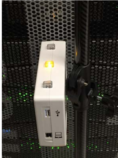
Figure 15. PurkayLabs: Awkward clamp fix (TH1 clamp placed on the rod clamp).
