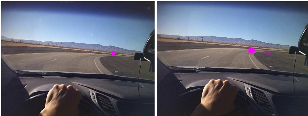
Figure 4.26: Eye-tracking showing far point (left) and near point (right) gaze points in driving.
