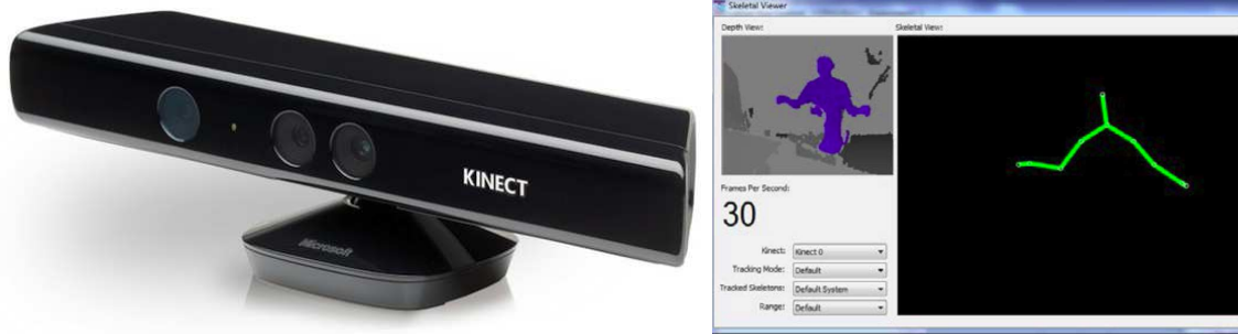
Figure 3.10: Microsoft Kinect sensor for skeletal tracking (left) and screenshot of real-time skeletal display during tracking (right).
