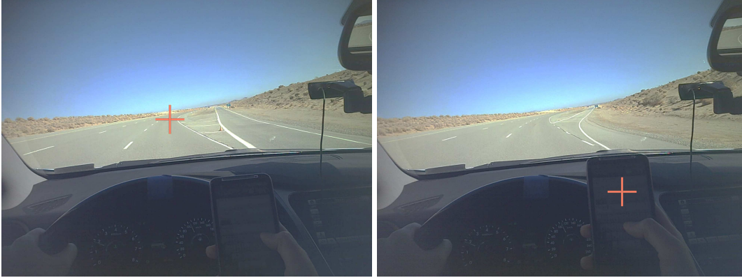
Figure 4.24: Measuring attention allocation in the distracted driving scenario through gaze fixations: (left) attention on the road and (right) attention on the phone.
