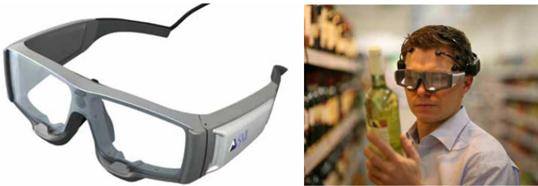
Figure 3.9: SensoMotoric Instruments head-mounted eye tracker [98] (left) and subject wearing eye tracker in an experiment [99] (right).
