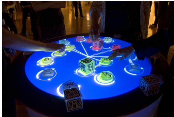
Figure 1.1: reacTable (2003-2010) is a multi-touch tangible interface for electronic music composition. Photo credit: Daniel Williams, © CC BY-SA 2.0, Created: 10 June 2007
