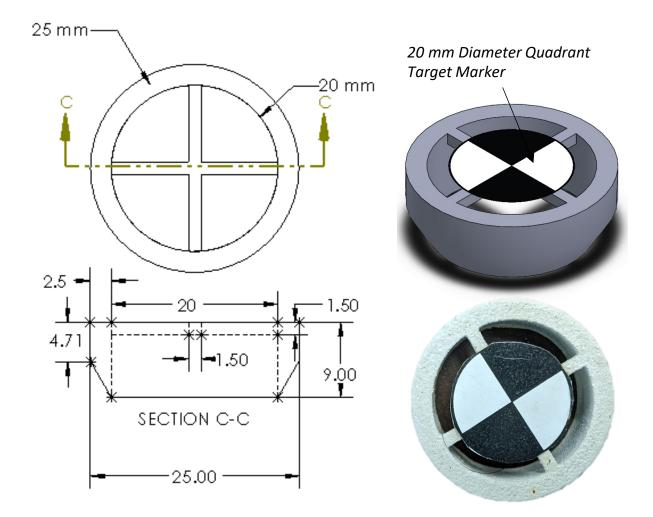
Figure 4.11. Drawings of the LEAP (Kutter B.L. et al. 2020) soil surface marker with a 15 mm diameter quadrant marker glued on its top (dimensions in millimeters).
