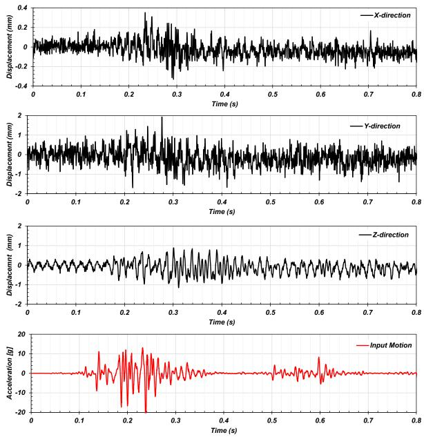
Figure 6.4. Movement of the centrifuge bucket with respect to the cameras in X-, Y-, and Zdirections during the first 0.8 seconds of shaking event EQM<sub>5</sub>.
