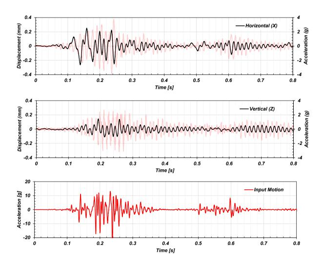
Figure 6.2. Computed horizontal (X) and vertical (Z) displacements (in black) of the Camera Beam obtained from the integration of the recorded horizontal and vertical accelerations (in red) by the accelerometers (CAMERA<sup>ACC H</sup> and CAMERA<sup>ACC V</sup>) placed on the Camera Beam.
