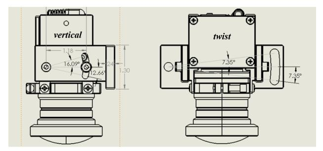
Figure 2.2. Adjustable camera angles using the available camera holder.
