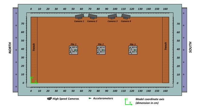
Figure 4.1. Centrifuge model test SKS03: Model plan view (dimensions in cm).
