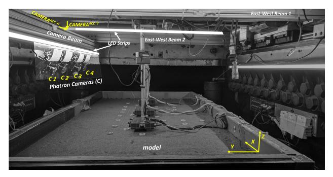
Figure 4.3. View of the completed model from North showing the four Photron cameras mounted on the camera beam.
