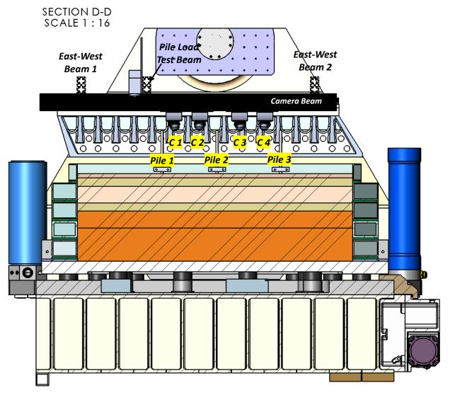
Figure 4.5. Cross-section view (at Section D-D in Figure 4.4) of the model container placed on the centrifuge bucket.
