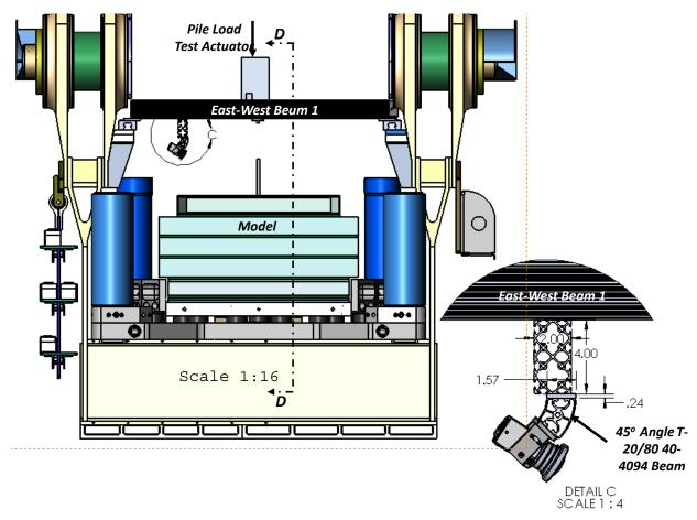
Figure 4.4. SolidWorks drawing showing the camera position and the camera mounting system (dimensions in inches).
