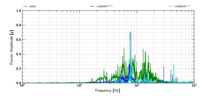
Figure 6.3. Fourier amplitude spectrum of the horizontal (CAMERA<sup>ACC H</sup>) and vertical (CAMERA<sup>ACC V</sup>) accelerations measured at the center of the Camera Beam compared to the input motion (BASE) accelerations measured at the base of the centrifuge container.
