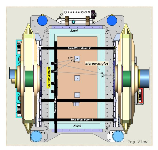
Figure 4.6. Plan view of the model container with the centrifuge bucket showing the locations of the Camera Beam, the East-West Beams, and the Photron cameras.
