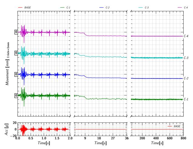
Figure 6.6. Movement of the container target markers in X-direction for shaking event EQM5.
