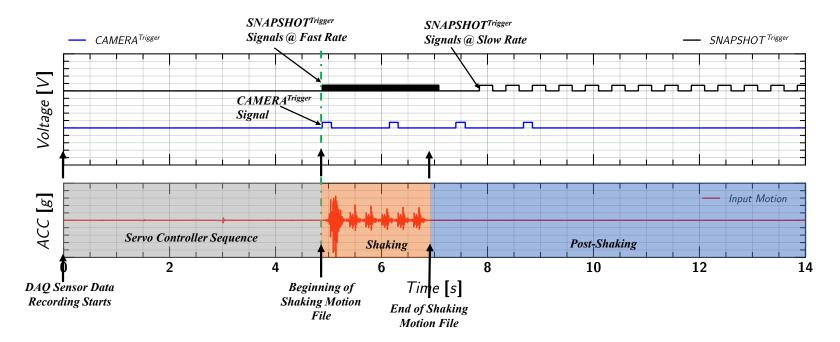
Figure 2.5. Illustration of external trigger modes (CAMERA<sup>Trigger</sup> and SNAPSHOT<sup>Trigger</sup>) used in the centrifuge model test SKS03.
