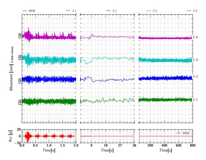
Figure 6.7. Movement of the container target markers in Y-direction for shaking event EQM<sub>5</sub>.
