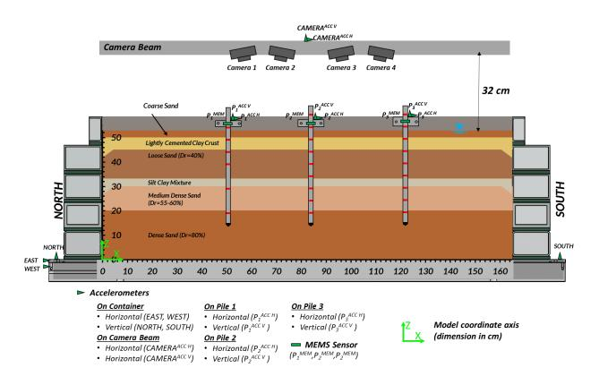
Figure 4.2. Centrifuge model test SKS03: Model cross-section view (dimensions in cm).
