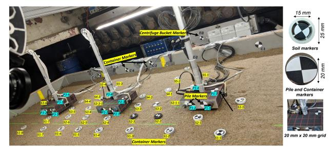
Figure 4.10. Camera target markers placed on the soil, on piles, and on the model container.
