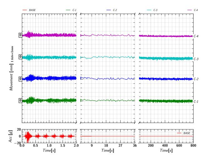
Figure 6.8. Movement of the container target markers in Z-direction for shaking event EQM<sub>5.</sub>
