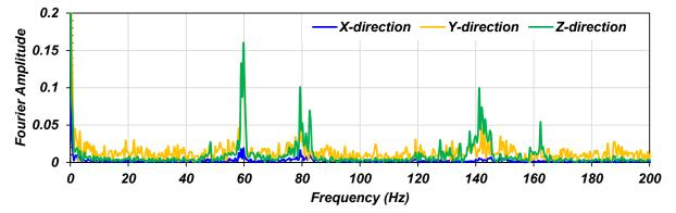
Figure 6.5. Fourier Amplitude of the displacements time-history in X-, Y-, and Z-direction of the centrifuge bucket marker F-0.
