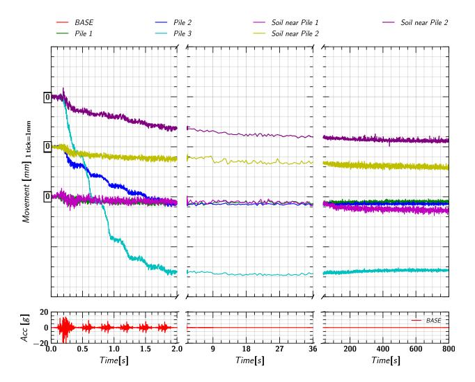
Figure 6.10. Settlement of the piles and the soil nearby for shaking event EQM<sub>5</sub>.
