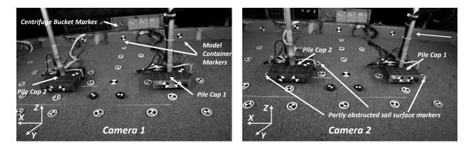
Figure 4.8. A view of the model from the North Pair Cameras (Camera 1 and Camera 2). The Xand Y- direction is in the plane of the soil surface whereas Z-direction is out of the plane.
