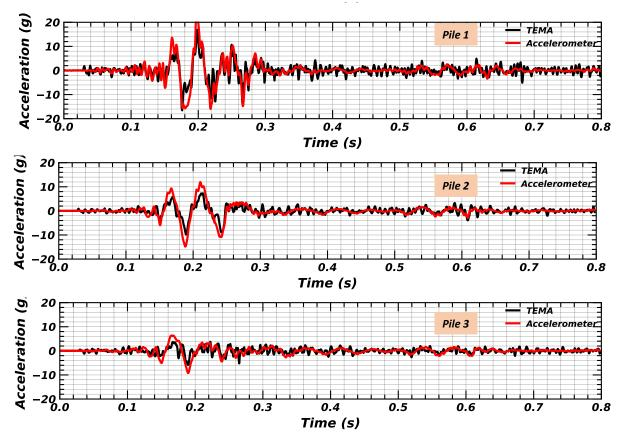
Figure 6.11. Comparison of horizontal accelerations measured from accelerometers placed on the pile head mass with the computed accelerations from displacement time-history measured from image analysis in TEMA for shaking event EQM<sub>5</sub>.
