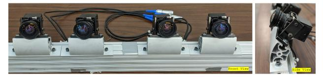
Figure 4.7. Front and side view of the four Photron cameras connected on the Camera Beam.
