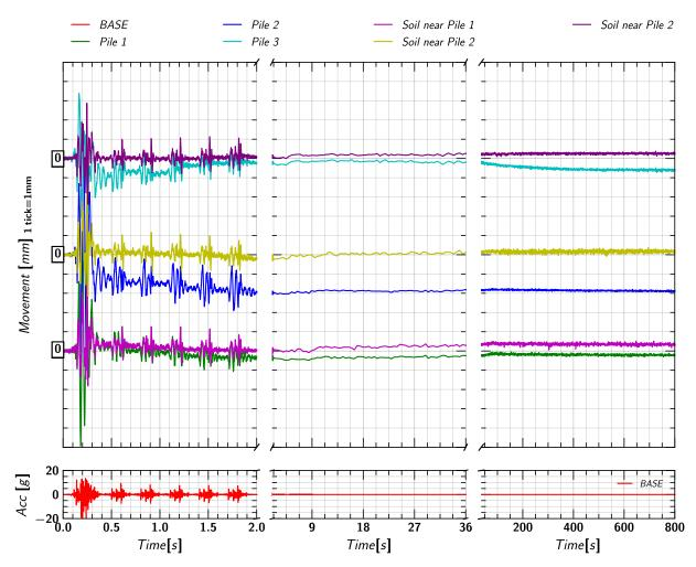
Figure 6.9. Movement in pile head mass and the soil nearby with respect to the container in Xdirection for shaking event EQM<sub>5</sub>.
