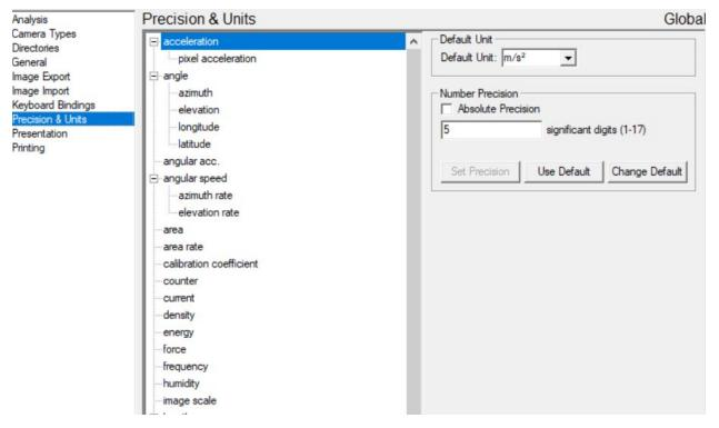
Figure 3.1 View of the TEMA settings window for setting up the units and precision of measurements while performing the image analysis.
