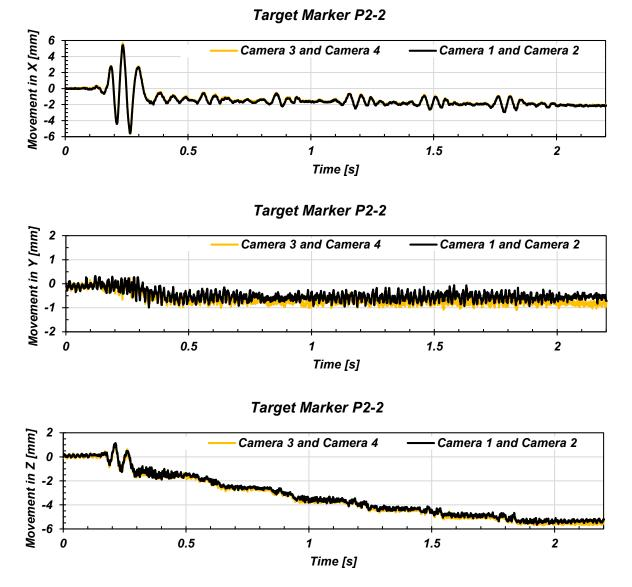
Figure 6.1. Measured 3D movement (relative to the camera) of pile 2 target marker P2-2 obtained from two separate TEMA analyses: one using the Camera 1 and the Camera 2 pair and the other using the Camera 3 and the Camera 4 pair.
