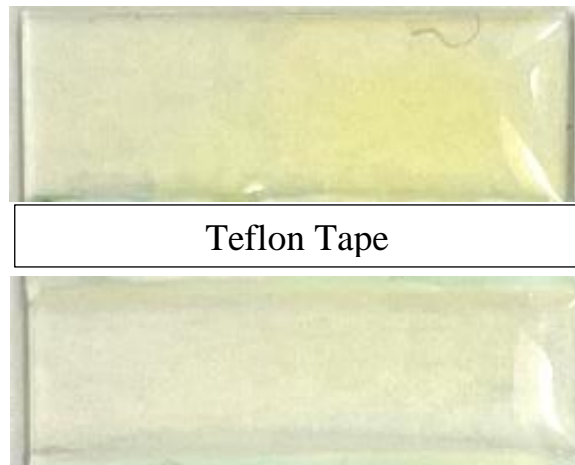
Figure 5-16 a) Photos of the color-forming complex. a) p24 antigen, detector antibody, streptavidin-peroxidase, and substrate b) p24 antigen, detector antibody, streptavidin-peroxidase, substrate, and stop solution. p24 antigen at concentration levels of 125 pg/mL (top) and 0 pg/mL (bottom) is immobilized on the glass slides.
