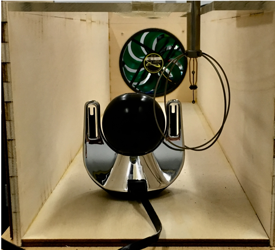
Figure 1. Purpose-built wind tunnel (81 cm x 18 cm x 18 cm) used to calibrate the thermal sensors in SAMBA
