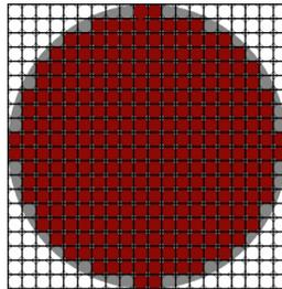
Figure 5. Lenslet geometry of our HS wavefront sensor. The gray circular area represents the image of the subject's eye pupil (diameter 6.675mm) and has a diameter of 10 mm. The dark red circles represent the position of the 284 "active" lenslets that are used during wavefront measurement.
