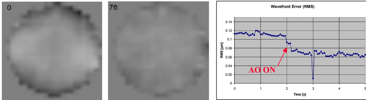
Figure 6. The ocular wavefront measured by the HS wavefront sensor before (left) and during (center) AO correction with the AOptix bimorph DM. Frame 0 is the first frame saved by the system; Frame 76 represents the wavefront measured 3.75 s after starting the archiving mode of our AO-control. Right plot shows total wavefront RMS error during AO operation. Lower values of the RMS at 3 s shows the RMS calculated during the blink.
