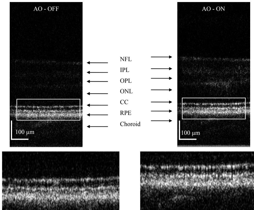
Figure 8. Upper images show B-scans acquired over 500 x1000 μm using AO-OCT implemented with the bimorph DM. Left image was obtained before AO correction and right image was obtained during AO-correction. Lower images show 2x magnification at the photoreceptor and RPE layers (100 x 400 μm). NFL – Nerve Fiber Layer; IPL – Inner Plexiform Layer, OPL – Outer Plexiform Layer, ONL – Outer Nuclear Layer, CC – Connecting Cilia, RPE – Retinal Pigmented Epithelium.
