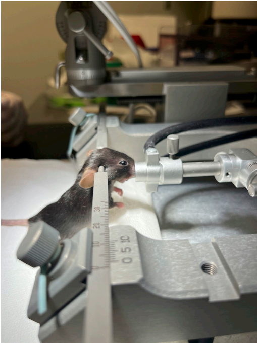
Figure 2. Final position of the mouse before CSF collection, in reference to step 17 “Fixation to Stereotaxic Instrument for CSF collection”
