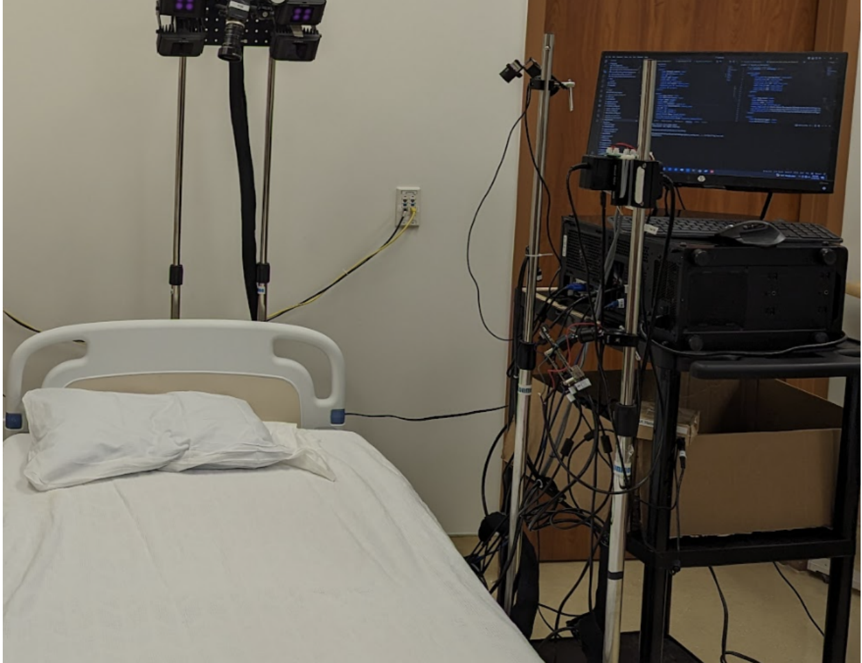
Figure 3.1: Our experimental hardware setup consisting of a thermal camera, a radar module, and data-processing auxiliaries located in a sleep lab. In this particular setting, we have placed the thermal camera and the radar to the right of the bed. Our setup also includes a microcontroller that is connected to the existing in-lab PSG hardware. This microcontroller sends pulse trains that can be used to synchronize the ground truth annotations with the captured recordings.
