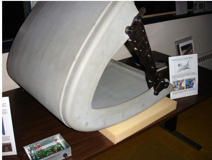
Figure 1-1. Blunt leading edge component used in the Space Shuttle. Typical radius of curvature at the tip is \sim 10 cm, made from SiC/carbon and carbon/carbon composites (adapted from http://www.pari.edu/shuttle-leading-wing-edge-web/ ).
