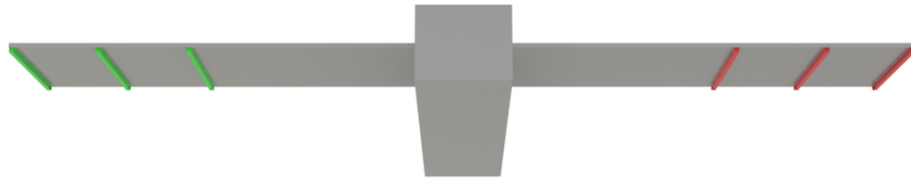
Figure 5.6: Perspective view of underwing lights perpendicular with leading edge of wing.
