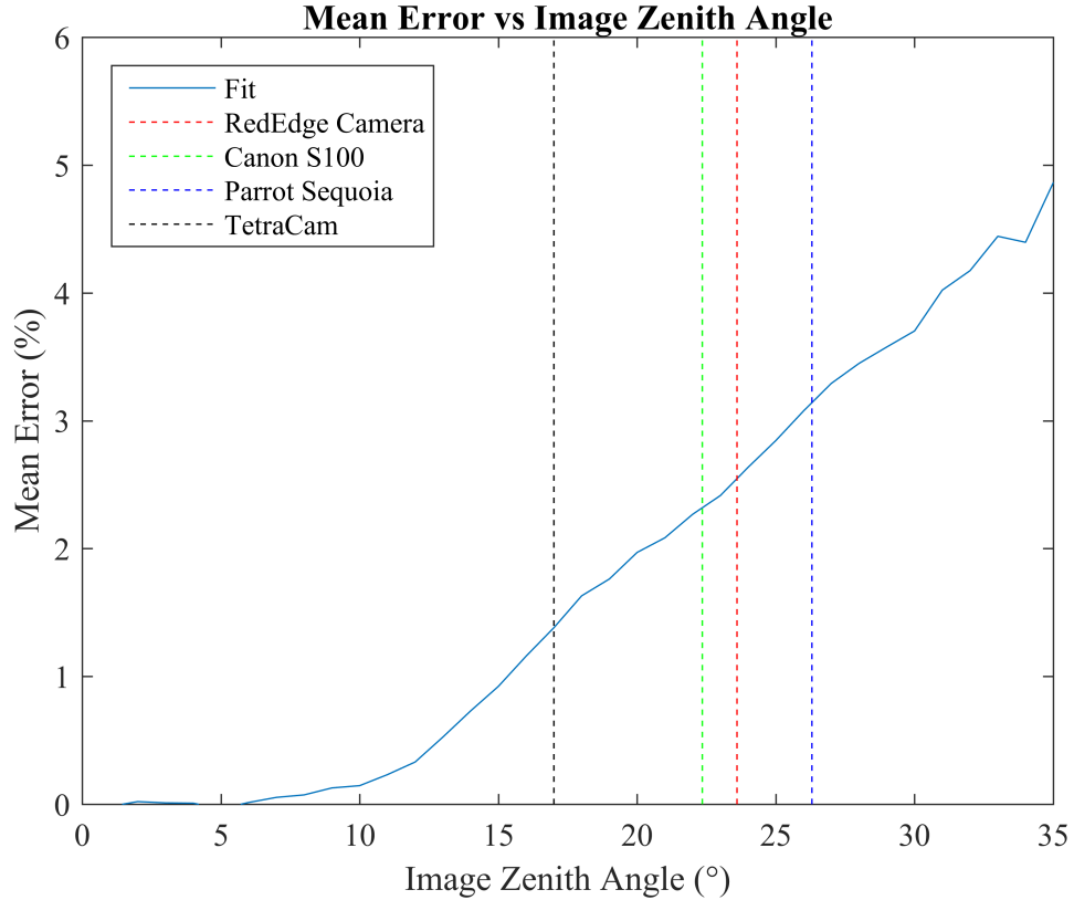
Figure 3.19: Mean error between satellite imagery and an increasing camera FOV. Common camera vertical FOV are provided as reference.
