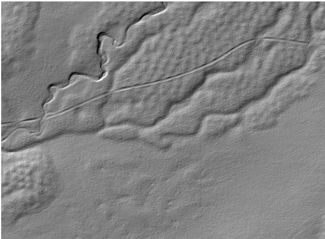
Figure 2.5: Example digital surface model with hillshade added for clarity.
