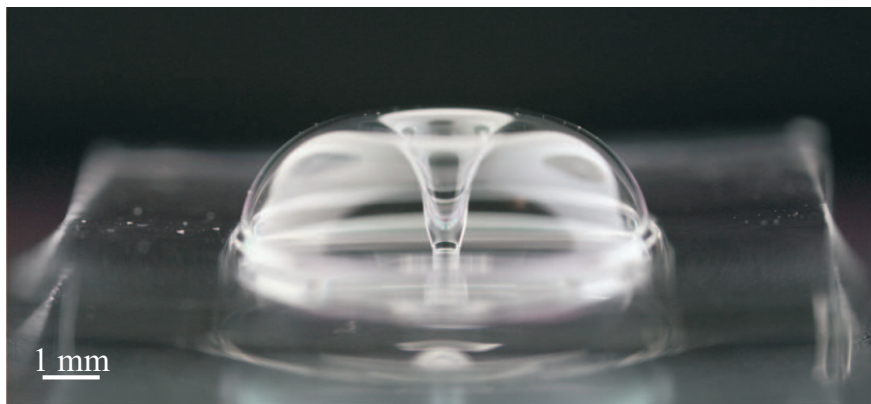
Figure 2.17: A 7 mm glassblown shell using reverse process with the device initial thickness of 175\ \mu\text{m} and the cavity etch depth of 325\ \mu\text{m} , as depicted in Fig. 2.16, on a device wafer with thickness of 500\ \mu\text{m} .
