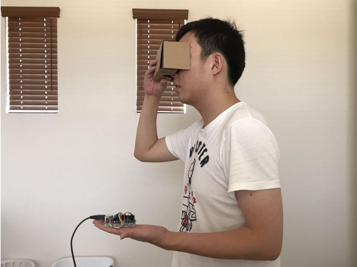
Figure 3.1c: Real-time motion simulating with MPU-6050 and Google Cardboard
