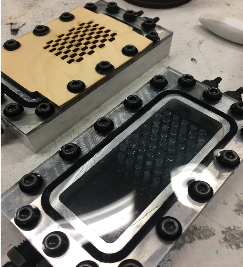
Figure 3.2: ‘Grated’ and ‘open-faced’ CORE Reactor lab prototypes
