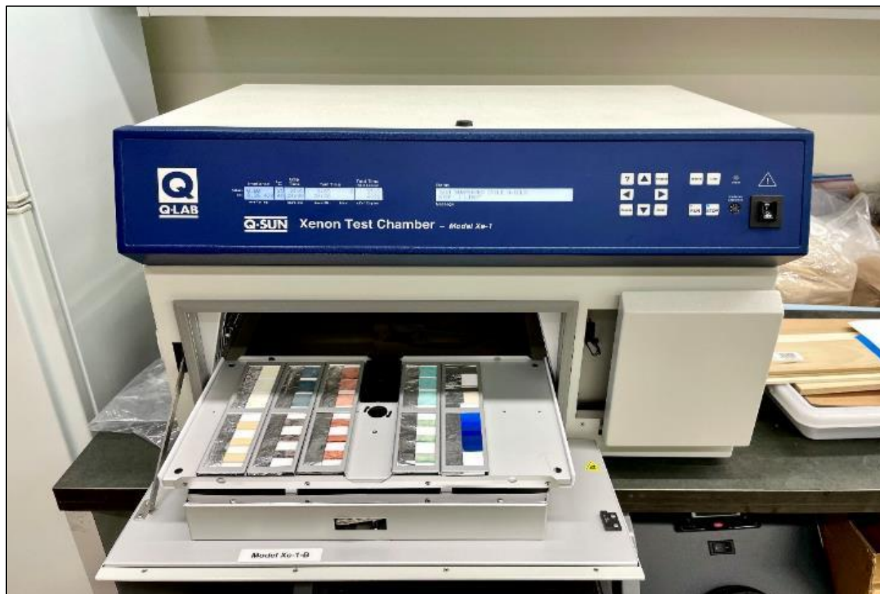
Figure 14: Fungal coupon pigments and ISO BWS, all half covered with aluminum foil, in the Q-Sun Xenon Test accelerating aging chamber.
