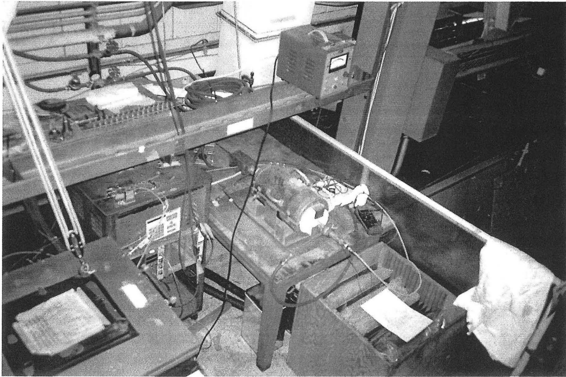
Photograph D.6: The MG, controller, and aerosol oven for the ^{266}\text{Bh} experiment.
