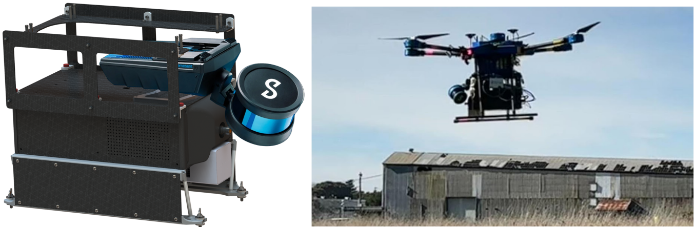
Figure 1: (Left) Rendering of the IVLAMP system. The rendering shows two mounting systems. The lower mounting system is used to attach the IVLAMP to the Spot robot, using four thumb-screws to attach to the Spot payload rails. The higher mounting system attaches IVLAMP to our UAV, using four screw points. (Right) A photograph of IVLAMP carried by our UAV at our UAV testing facility in Richmond, California, USA. Note, in this photo, the Spot mounting system is not present.
