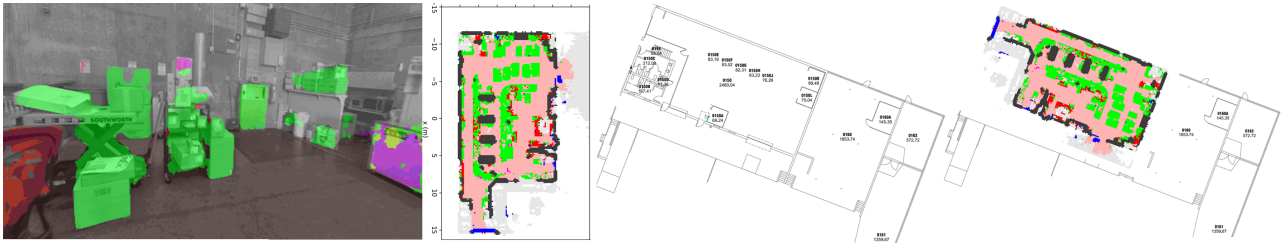
Figure 5: From left: (1) A semantically labelled imaged, (2) a floor plan derived from a series of labelled images projected into the 3D model and aggregated, (3) actual floor plan (4) floor plan with semantically-derived floor plan overlaid.
