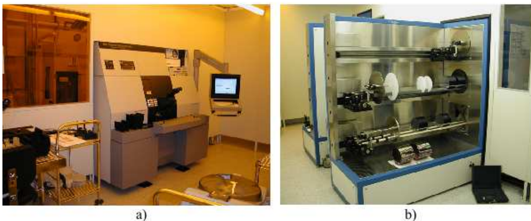
Figure 10: Photographs of processing equipment at the LBNL MicroSystems Laboratory. a) Photograph of the projection aligner used to print patterns on 150 mm diameter wafers. b) Photograph of high-temperature furnaces used to oxidize silicon, deposit thin films, and anneal 150 mm diameter silicon wafers.
