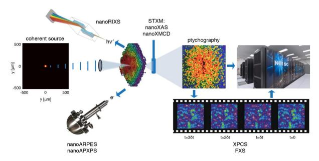
Chemical imaging experiments at the ALS have recently achieved few-nanometer spatial resolution in 2D on a model material, but on a more typical, realistic object can provide only 15 nm resolution with limited spectral coverage and temporal sensitivity. The upgraded ALS, on the other hand, will allow spectroscopies like angle-resolved photoemission spectroscopy to be
