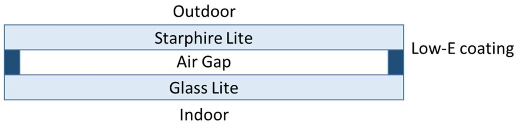
Figure 3 Schematic diagram of the Low-E reference IGU
