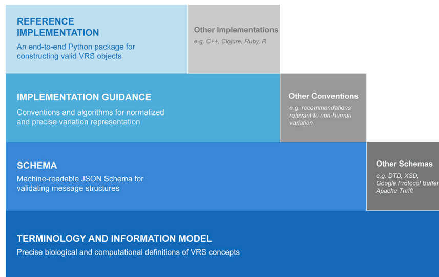
Figure 1. Components and extensions of the Variation Representation Specification
