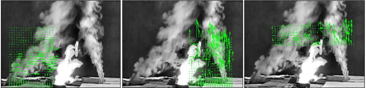
Figure 4-10: Outer (left), inner (middle) and upper (right) plume instantaneous velocity fields from OpenPIV processing
