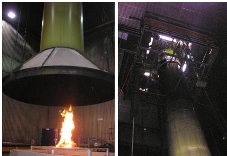
Fig. 1. a) Fire under laboratory flue, b) Looking up at instrumentation platform
