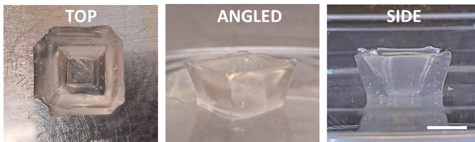
Figure B25: Different angles of 3D printed inverted pyramid showcasing overhanging layers and sharp corners (scale bar: 4 mm).
