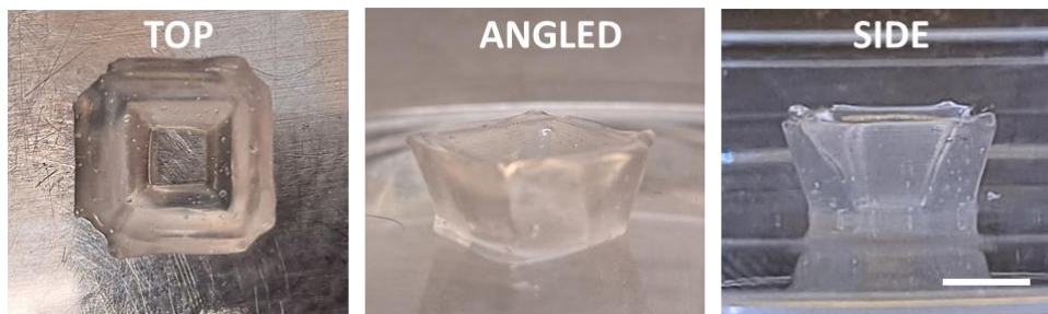
Figure 3.13. Different angles of 3D printed inverted pyramid showcasing overhanging layers and sharp corners (scale bar: 4 mm). 52 Reproduced with permission from John Wiley & Sons Inc.
