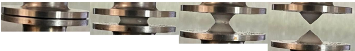
Figure A27: Time lapse images of 20wt% hydrogel capillary thinning and breakup between parallel plates.
