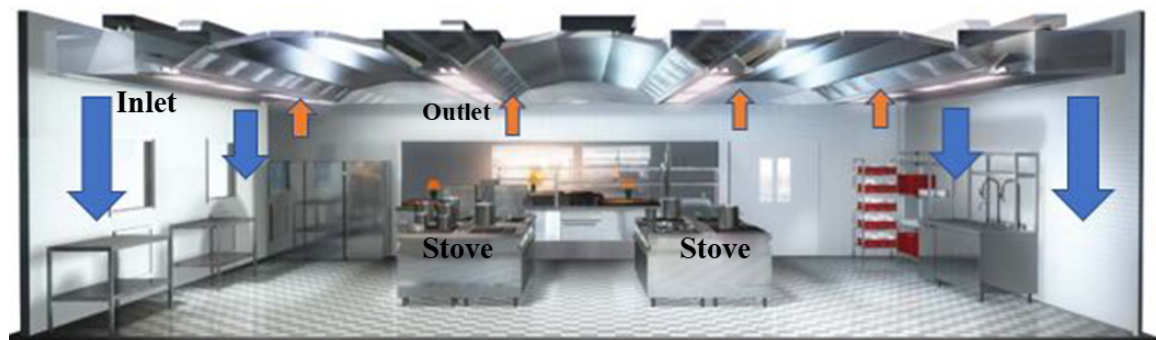
Fig. 24. Ventilated ceiling with air curtain ventilation.
