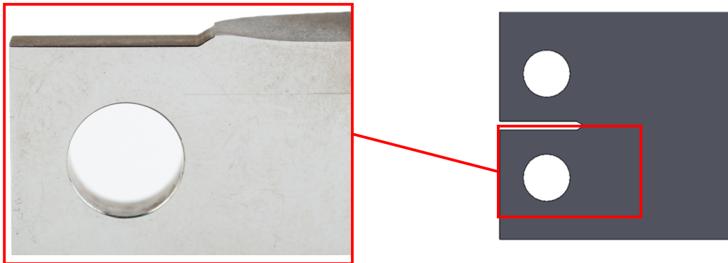
Figure 5.8: Photograph of twisted crack path of PBF-L2 -M (V). Location in the specimen indicated by the red box.
