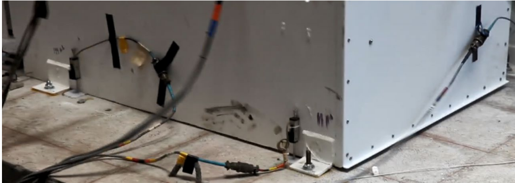
Figure 25. Uplift of the component attached to concrete.
