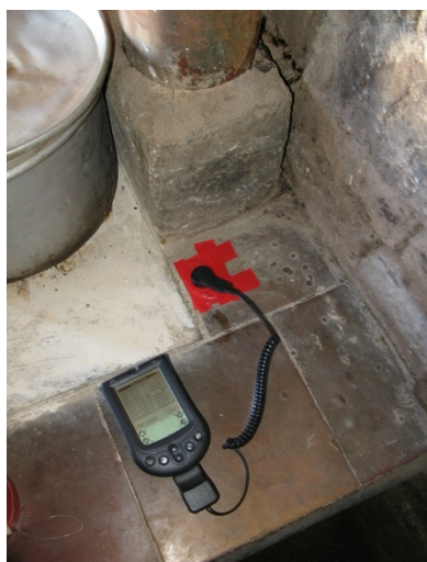
Figure 3.4 Small temperature dataloggers were used as Stove Use Monitors (SUMs). The SUMs, attached to the chimney-stove body, were programmed bi-monthly in the field and the data were downloaded using PDAs.
